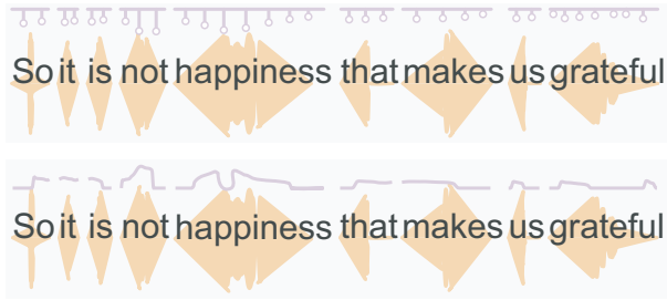
Fig. 5. Design alternatives for encoding pitch values, including a music note design (top) and the final design used in SpeechLens (bottom).
