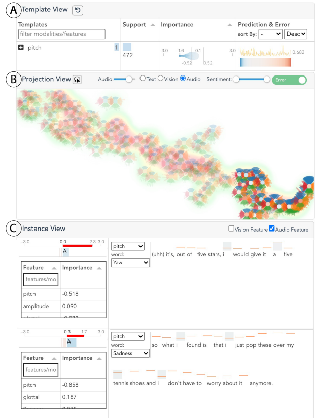
Fig. 7. Negative influences of voice pitch. A: “pitch” is the most frequent acoustic template, and it always has a negative impact (as indicated by the dots in the bee swarm plot). B: The selected group of instances with large pitch values (as indicated by the large radius of the blue sectors). C: Two high-error cases where the model captures the turning points of the pitch but wrongly associates pitch with negative influences.
