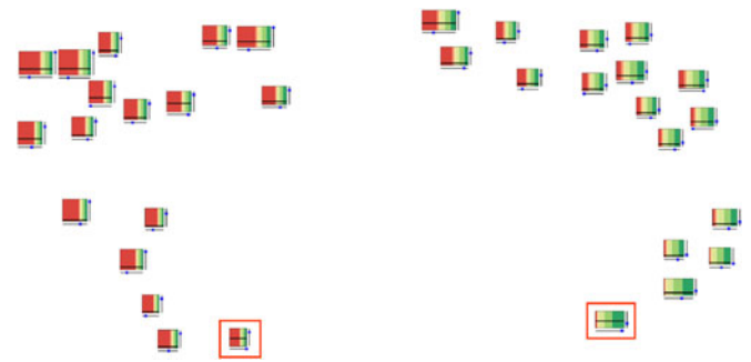
Fig. 5. Overview. The graph is used to show the similarity among peaks. Each node represented by a glyph corresponds to a peak. The layout of the graph is calculated by multidimensional scaling based on peak similarity. A short distance indicates high similarity between two peaks.
